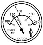
Figure 49. Coolant Temperature Gauge
